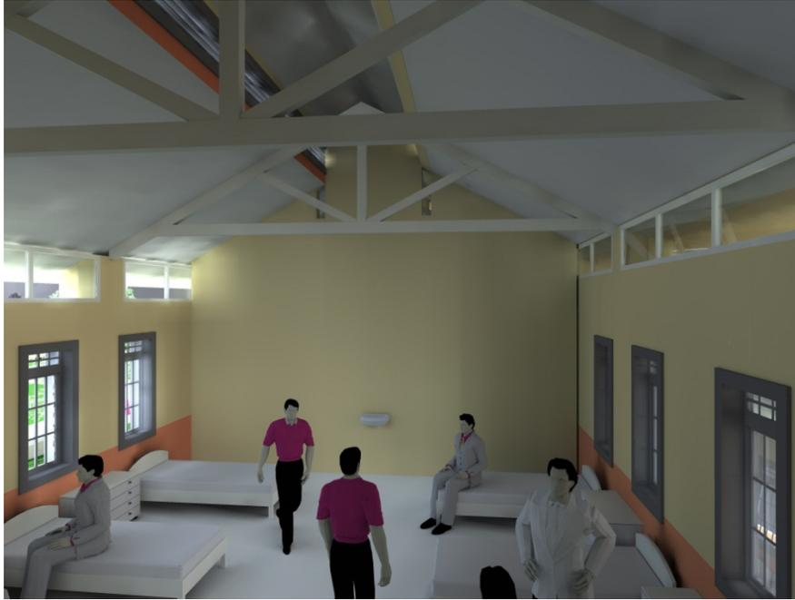
**Ridge ventilation proposed inside male ward existing clerestory windows are maintained by replacing the old wire meshes**
