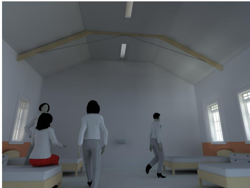
Ceiling louvers proposed inside female ward. These louvers enable ventilation of the wards via raised ridge ventilation
