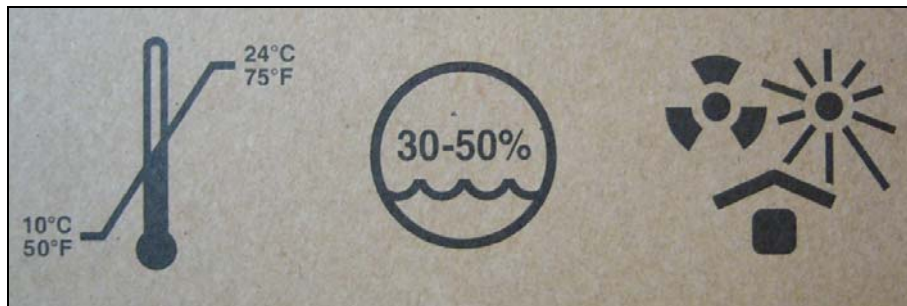
Figure 2.11 Sample X-ray film box indicates storage condition
