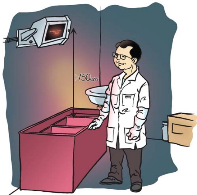
Figure 2.9 The distance between safelight and developing tank
