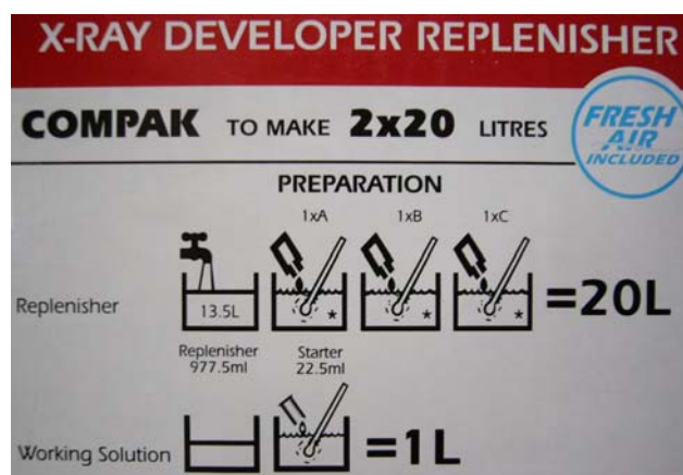
Figure 2.15 Sample instructions for preparation of developing solution
