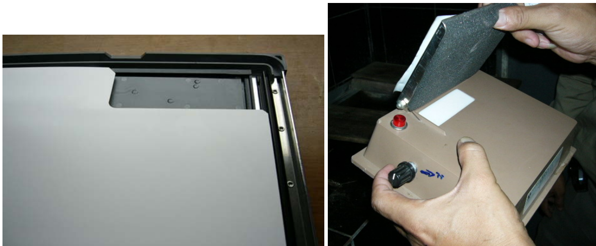
Figure 3.5 Special X-ray cassette (left) and simple identification printing device (right)
