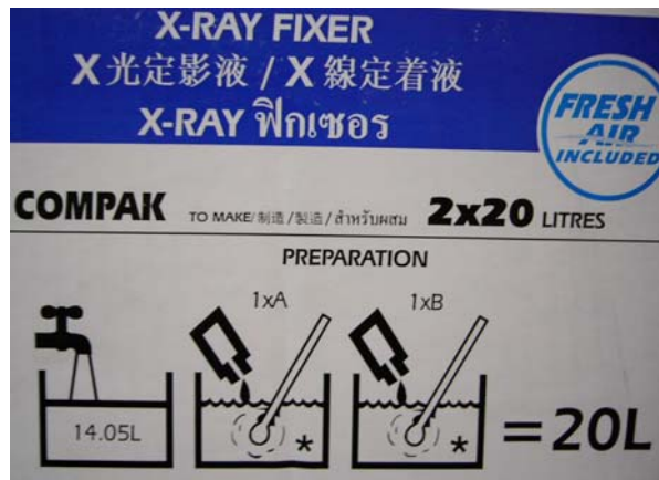
Figure 2.16 Sample instruction for preparation of fixing solution
